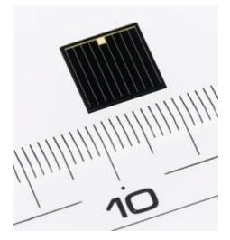
Sharp's 37.9 percent efficient III-V solar cell
