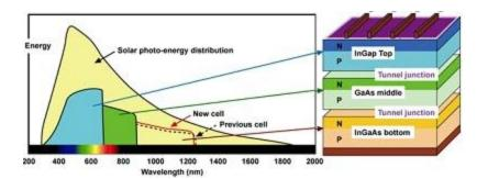
Structure of Triple-Junction Compound Solar Cell
