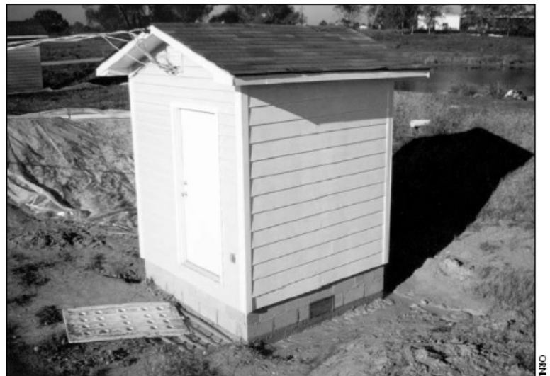
Because reproducing flood conditions in actual houses was not practical, we made small prototype test structures.
